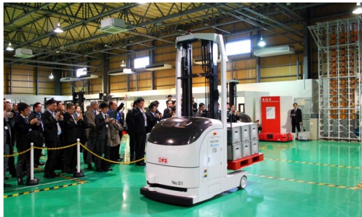
Demonstration of Platter Auto laser-guided AGF model (Onsite Training Center)
