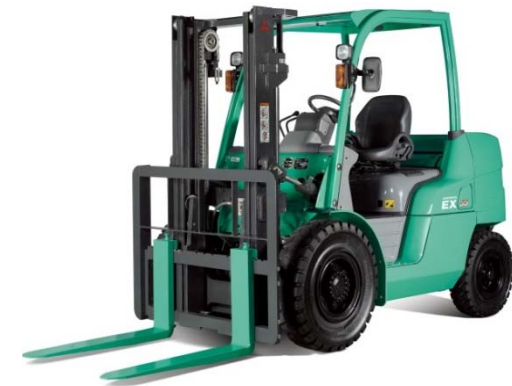
Diesel engine-powered forklift for Japan "GRENDiA EX" (3.5t-5.5t) compliant with Tier 4 emission regulation for non-road diesel engines.
