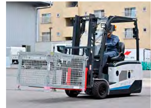
Fuel-cell-powered forklift truck undergoing demonstration testing
