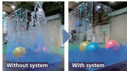
Vibration and shock absorption rate with Good Running System
