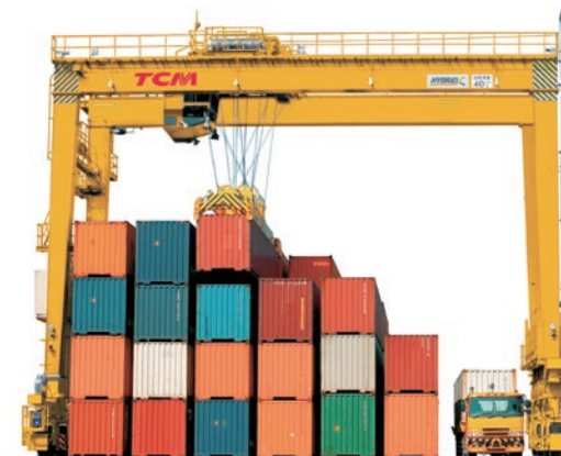
Rubber-tired gantry crane
