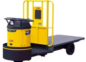
Eletruck turret truck equipped with Li-ion battery
