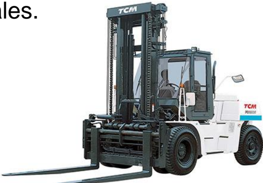
Forklift with large diesel engine (10-16 t) for Asian market
